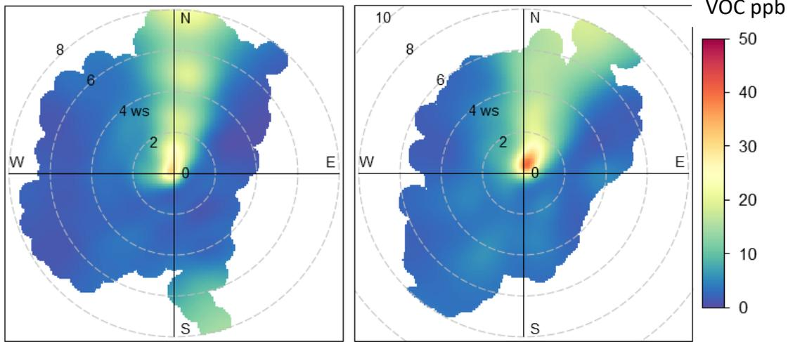
SPods provide wind and VOC data on source direction
