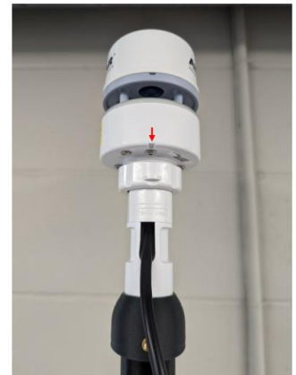
Install MET ( Notch must point North)
